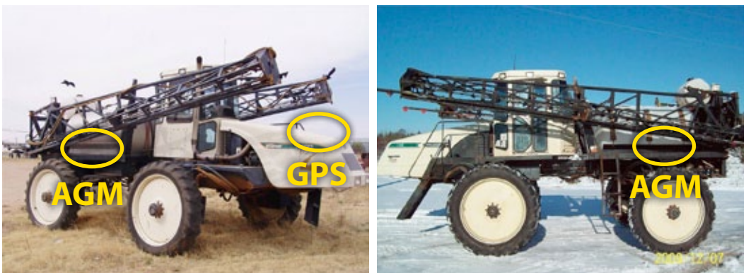
Figure 1-13: Recommended Electronics Installation
