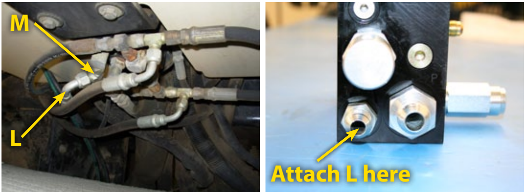
Figure 1-8: Install Tank Adapter and Hose
