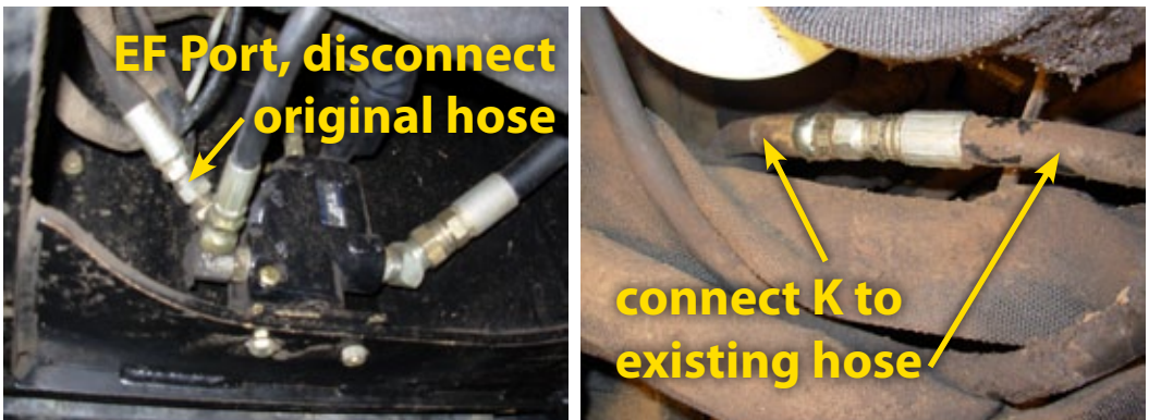
Figure 1-7: Install Pressure and EF Hoses
